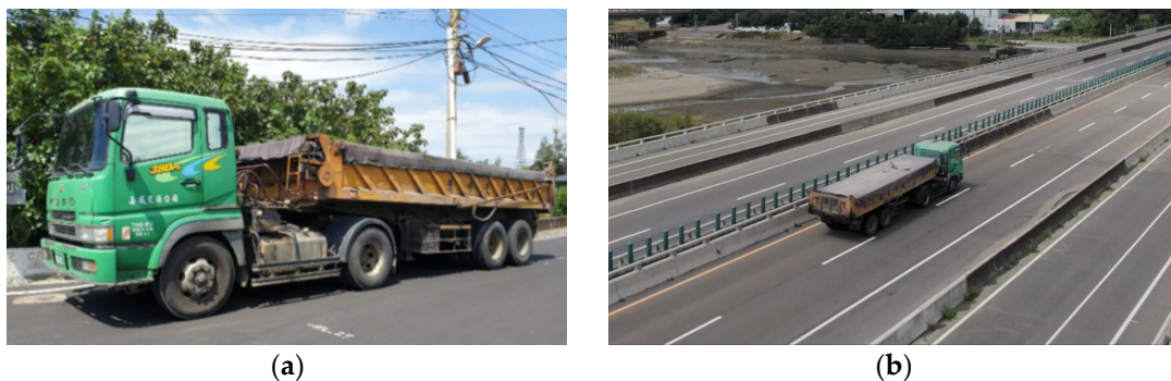
Figure 16. Vehicle loading test: (a) image of the vehicle, which weighed 38.46 metric tons, and (b) photo of the vehicle when it moved on the bridge.
